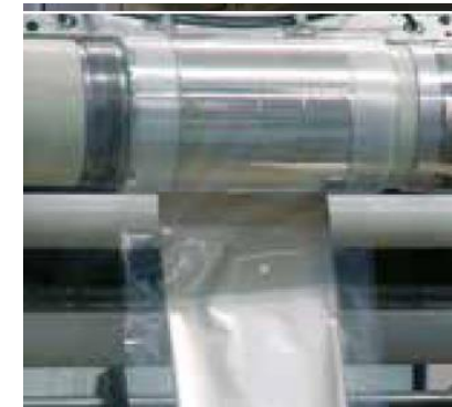
Li on Cu foil via vacuum deposition process (sidrabe.com)
