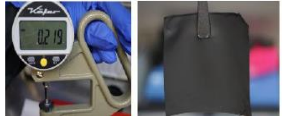
Dry film solid state cathode (0.1 wt% binder content)
